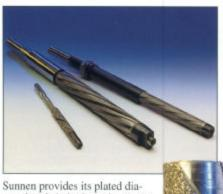
Sunnen provides its plated diamond tools in both steel and cast iron sleeves and with standard and special purpose cutting surface sculptures. Cast iron sleeves (shown above) are specially designed and allow for deeper fluting, offering advantages over the competition: greater oil flow; better chip removal; better cutting/bore geometry.
