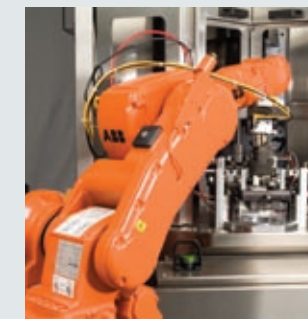
A TWO-AXIS OR MULTI-AXIS SERVO ROBOT CAN BE INTEGRATED INTO A SUNNEN MODULAR HONING SYSTEM.
