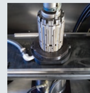
INTEGRATED AIR SIZING SYSTEMS CONTROL THE ACCURACY OF BOTH ROUGHING AND FINISHING PROCESSES.
