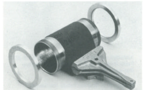
KKN-700 Universal Honing Fixture, HF-300 Workholder, and two loose-fitting End Caps used to fixture Cylinder
